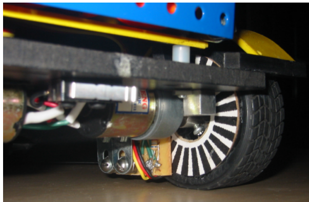
Figure 5: Reflective IR sensors mounted on a bracket inside the left drive wheel
