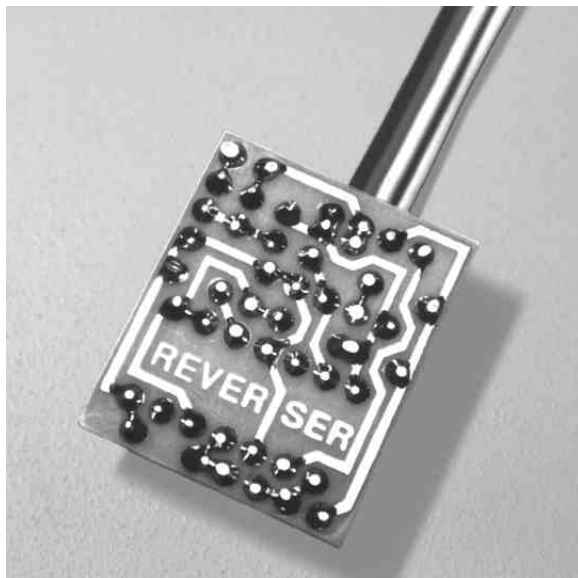
Fig. 8 Photograph of the assembled servo reversing circuit from the trace side of the printed circuit board.
